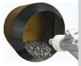
Sandblasting machine for cleaning sandblasting deburring of small parts in rotating basket.
