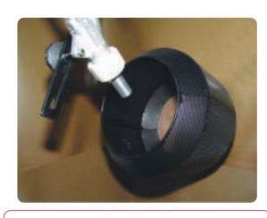
Drum is available in diameter of 300 mm, depth of 250 mm and load capacity of 10 kg. Blasting gun is movable and allows different types of nozzles.
