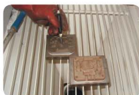
Delicate cleaning with injector blast gun
