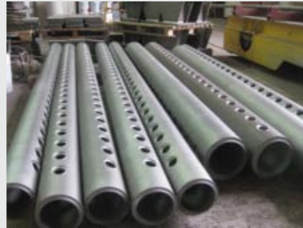
The protective cover enables sandblasting of perforated tubes.
