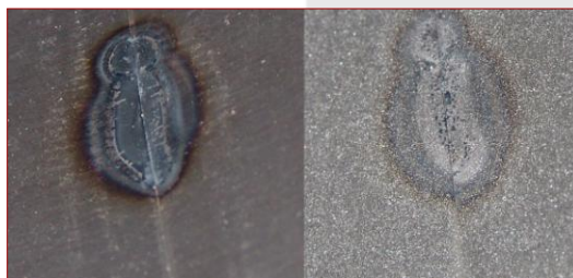
Example of welded sheet metal before and after sand blasting with steel grit.
