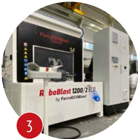
Recipe Control Touchscreen interface with diagnostics, media control, pressure, timing, and motion.
