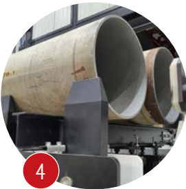
Automated Unloading Station finished pipes are ejected to a soft-end ramp or exit track, ready for next operations.
