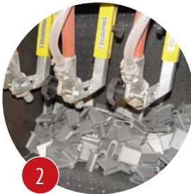
Oscillating Blast Guns Three to four nozzles sweep across the batch using programmable oscillation.
