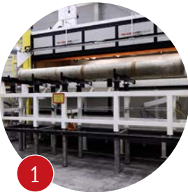
Automated Pipe Loading Ramp Pipes loaded from forklift or conveyor and load them onto support fixtures.
