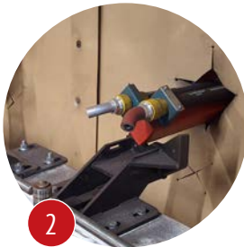
Servo-Driven Manipulator Precise internal lance moves axially through the pipe for full 360° internal coverage.
