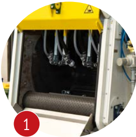
Rotating Tumble Belt Rubber belt gently rolls parts for uniform blasting.
