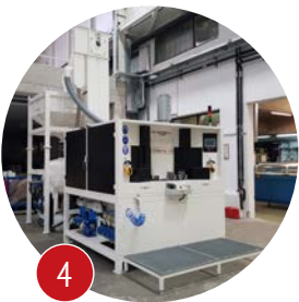
FerroSmartPanel Integrated PLC/HMI with recipe selection, diagnostics, and remote access.
