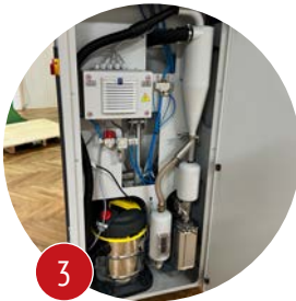
Integrated Media Recycling Cyclonic recovery system with vacuum filter allows efficient re-use of media
