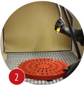
Manual Pressure Blasting Powerful and precise blasting using foot-pedal control and pressure pot system.
