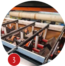
Adjustable Roller Fixtures Pipes are clamped and rotated to match diameter and blasting pattern.
