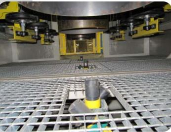
Usually water heaters are rotated and blasted with special nozzles with vertical movement. If needed, rotating nozzles can be used.
