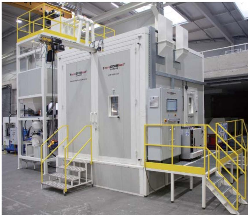
The FerroECOBlast ASP1000 ECO automatic robotized peening cell
