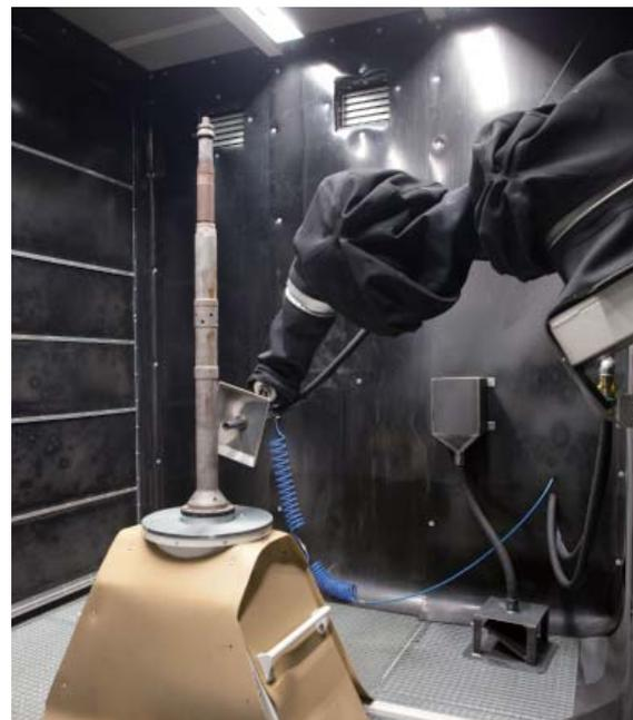
Inside the FerroECOBlast ASP 1000 ECO shot peening cell
